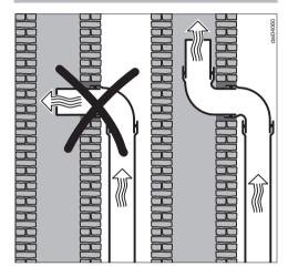
Where ducting is horizontal, it must be laid to slope away at at least 1 cm per metre.
